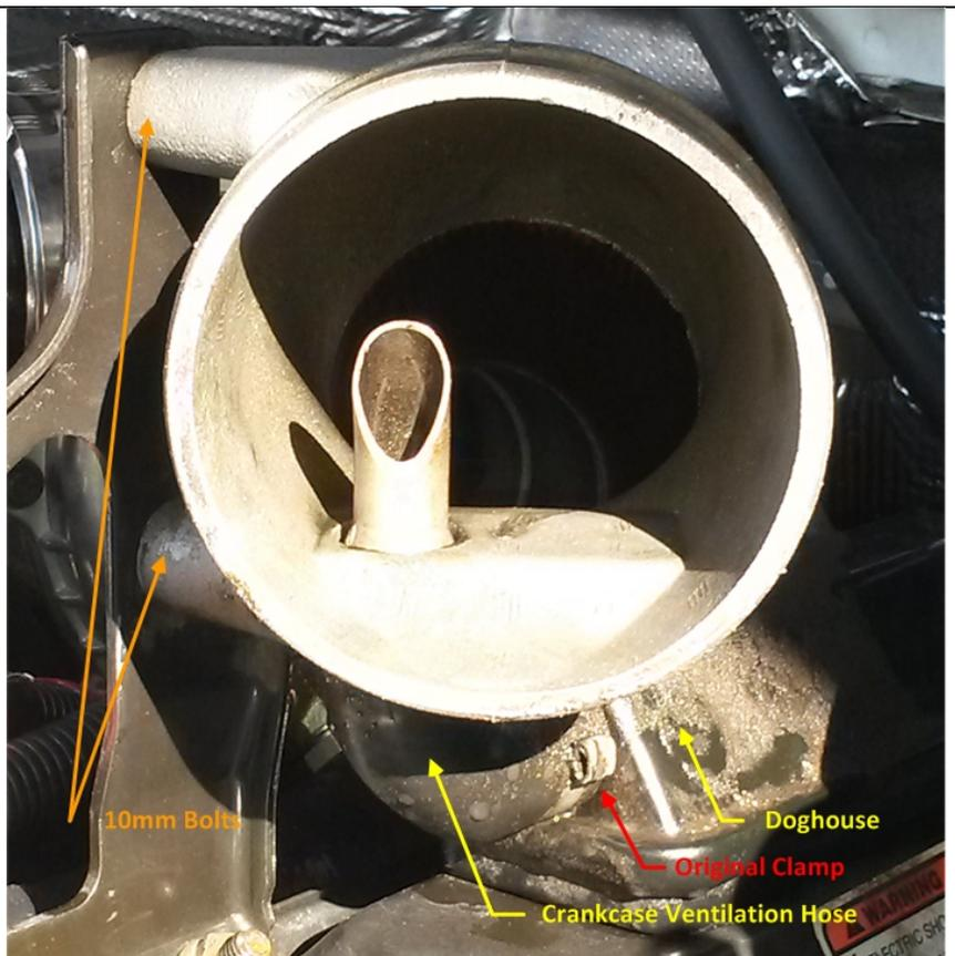
3. Remove the two Phillips head bolts holding the doghouse in place on the driver side valve cover. Lift the doghouse off the valve cover.
