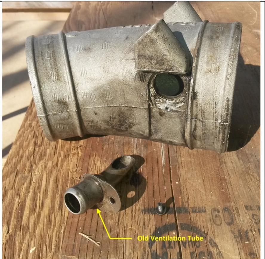
10. Measure the recessed opening in the aluminum intake tube. Cut the aluminum plate to cover the opening in the aluminum intake tube. Let the plate extend approximately  $\frac{1}{2}$ " past the threaded bold hole.
