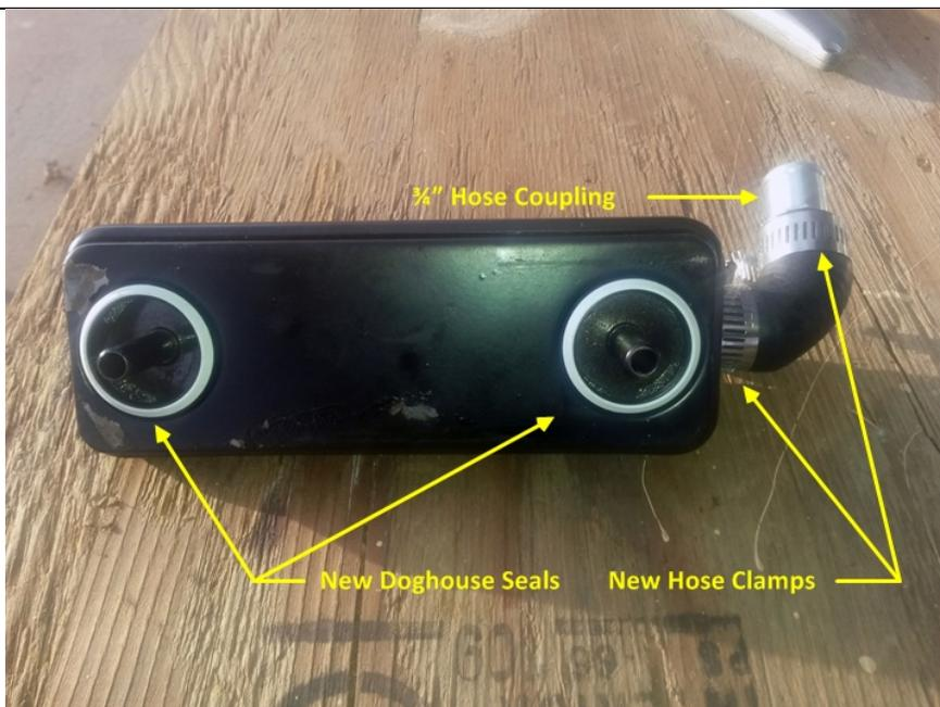
6. Rotate the doghouse 180° from the original position and re-install on the valve cover.
