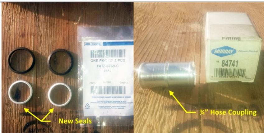
5. Replace the factory hose clamp on the crankcase ventilation hose with a 3/4" hose clamp. Insert the 3/4" hose coupling and install a 3/4" hose clamp. Do not completely tighten the hose clamps at this time.
