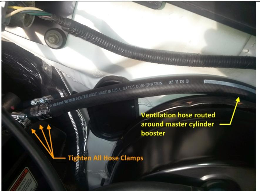
8. Secure the new ventilation hose to the frame rail. Trim off the excess length of the ventilation hose.
