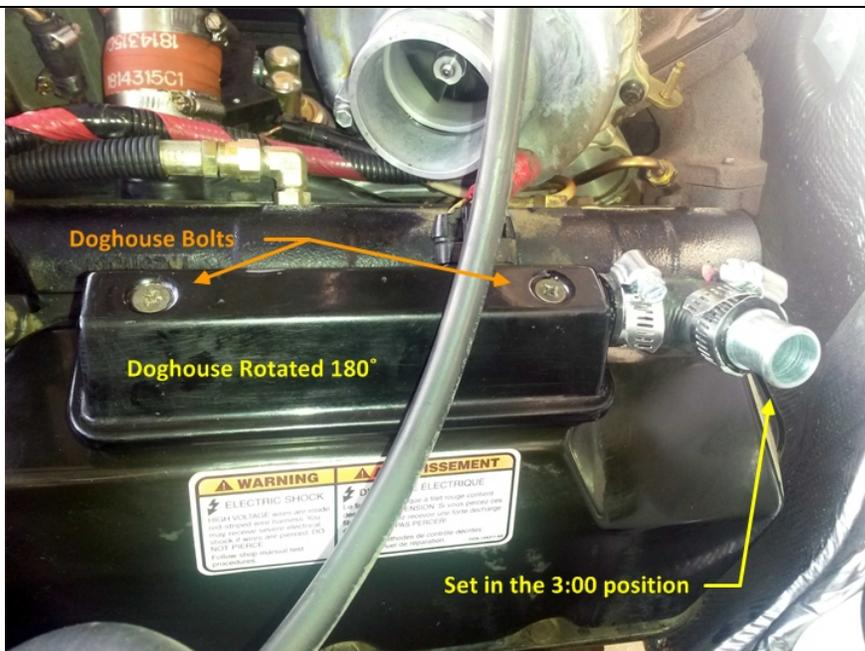
7. Route the new ventilation hose around the master cylinder booster and down between the inner fender and the firewall to the frame rail. Slide a hose clamp onto the new ventilation hose. Slide the new ventilation hose onto the  $\frac{3}{4}$ " hose coupling. Tighten all the hose clamps securely.
